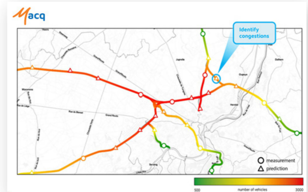
Figure 1: The principle behind traffic interpolation. Estimates of traffic metrics are provided at different locations on the network (triangles) based on real-life measurements from sensors (circles) used during the training phase of the interpolation model.
